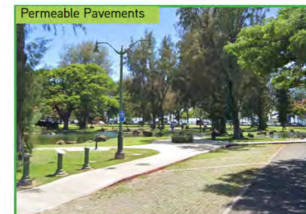
Permeable Pavements Capture water in place while filtering it and potentially replenishing aquifers Source: Google Maps, "Street View Kapiolani Park", Honolulu.
